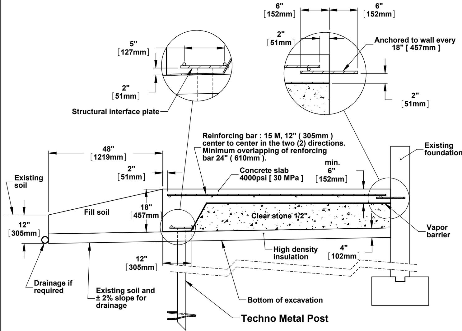
**Note :** Be aware that it is your responsibility to adequately protect the concrete slab on ground against freezing and it is important to drain the concrete slab, in order to avoid any movement of rising ( concrete slab and the Techno Metal Post ) during the period of freezing-thawing winter.
