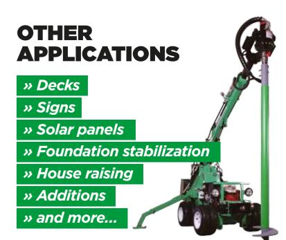
Our exclusive green polyethylene sleeve protects the piles from soil movement.
