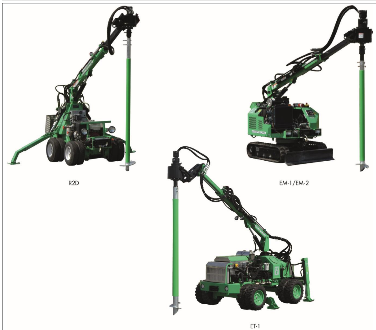
Figure 8 Machines for the installation of the Techno Metal Post (outside the scope of this Certificate)
